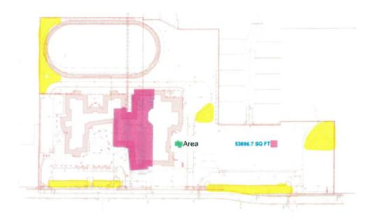
The recommendation of the architect, civil engineer, and the soils testing company is to remove the soil and then replace it with a structural fill material. As this problematic soil was a "unknown" condition at the time of bid, it qualifies for a change order.
